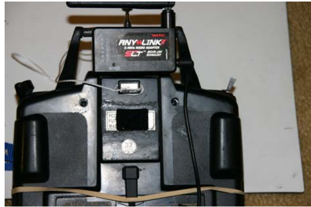
Installed using the TX handle for Stability, a Velcro mount could also be used. Note the Trainer cable plug in and also a string attached to the crystal so it wont get lost.
