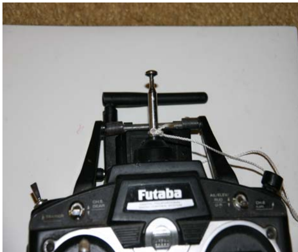
Front view – The FM tx is still useable, just unplug the training jack
